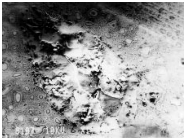
Fig. 5. SEM photograph of the sample exposed for 15 minutes duration with beam intensity of 50 mW.
